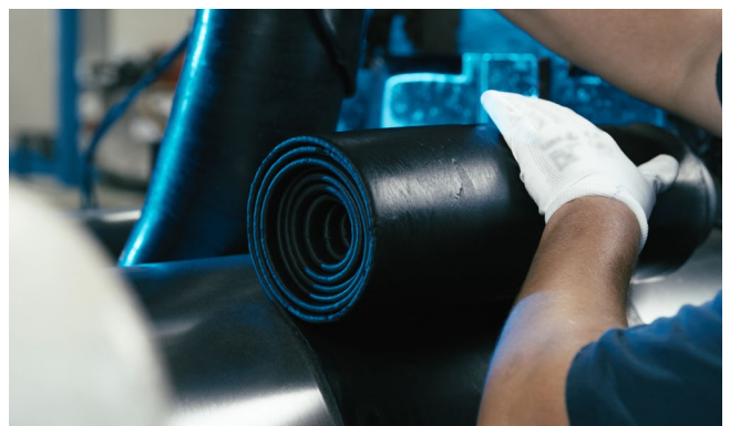
Rubber material moving through a calendering process to form rubber sheet.
