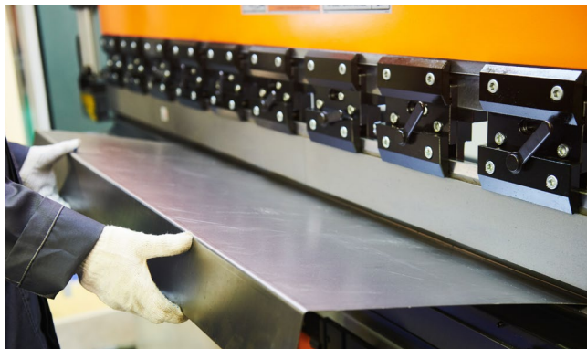
Metal Engineering Process Worker operating a hydraulic steel plate bending machine.
