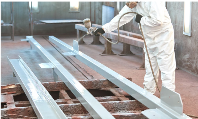
Powder Coating Technician sprays powder paint from a gun on metal products.
