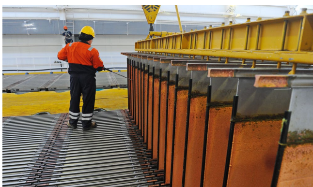
Factory Worker washes plates of cathode copper to make copper wire, cable, sheets, tubes, and alloys.
