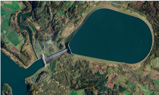
Pumped hydroelectric facility to generate power by leveraging gravity and water turbines.
